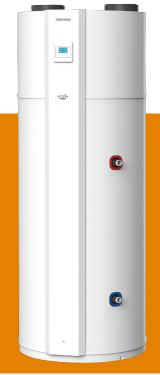
Air/water heat pumps in monobloc design for heating process water to +65°C. Compact unit for indoor installation in two basic versions with integrated 190 or 260 liter water tank. Flexible connection options for supply air and used air, connection to Modbus possible as standard. Variants available for integration of photovoltaic or thermal solar system via additional heat exchanger.
